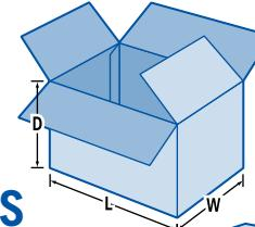
Shipped flat by the single unit. Seal with tape, glue or staples. Used for air and truck freight consolidation. Meets all Domestic and Air Transport Association standards. Both outside and inside dimensions are listed.
