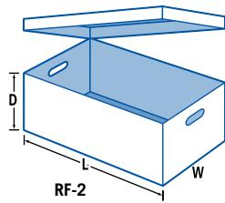
Shipped in flat unitized bundles for quick, easy assembly. No tape required. All dimensions are inside dimensions.
